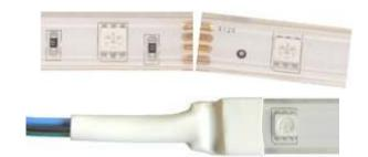
Be careful when soldering that you do not overheat the pads as this heat can damage the pad and the LEDs, a small dab of flux paste helps with a fast solder connection. **Make sure the wire you use is rated for load.**
